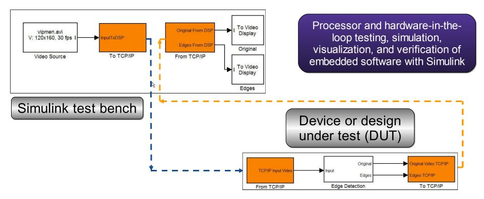
Simulink system design embedded on DSP
