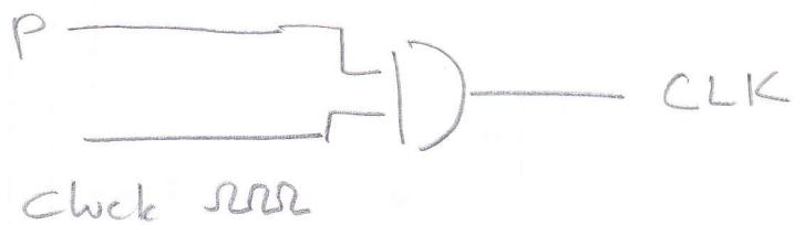
This signal will be used to clock the counter.
